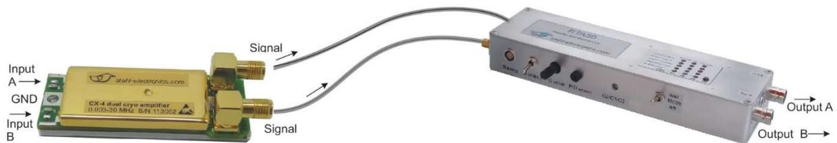
Fig. 4: cabling scheme of connecting the differential version of CX-4 to room temperature controller/post-amplifier.
