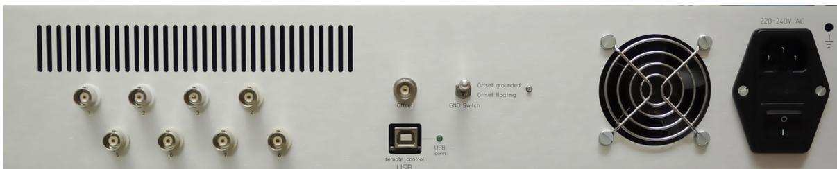
The rear side (8-channel device with rear outputs is shown) features a row of output channels (BNC) and a reference floating ground input, in case this option is installed. The galvanically isolated USB interface connects to a control PC.
