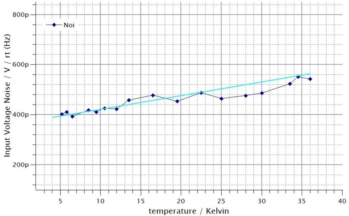
Fig. 15: Voltage input noise density at  $f = 1.5\text{MHz}$  as function of ambient temperature
