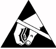
This device can be **damaged** by ESD (Electrostatic Discharge). It is **strongly recommended** to handle the device with appropriate precaution. Failure to observe proper handling and installation procedures can cause serious damage. This ESD damage can range from subtle performance degradation to complete device failure.
