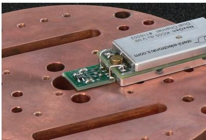
hole at the input (see photo) may serve as central connection point, to which the signal ground may be connected. All lines from the signal source to the amplifier's inputs should be kept as short as possible and of low inductance-style (no large loops or spirals).
