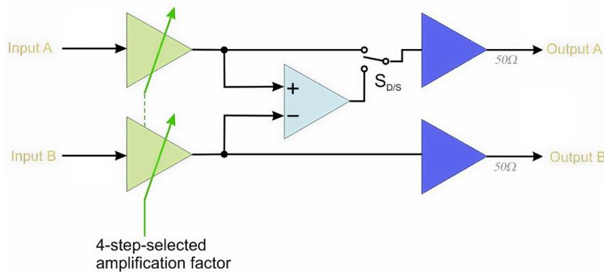
Figure 6: Schematic diagram of the analog signal amplifier circuitry inside the roomtemperature controller. The mode switch  $S_{\text{Dual/Differential}}$  allows for choosing between dual-channel or differential operation
