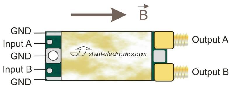
Fig. 2: Solder Pad Input Connections, SMA connectors
