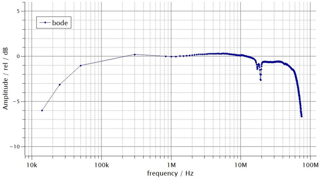
Fig. 11: Amplification at cryogenic temperature (6K) as function of frequency, expressed in dB relative to the amplification factor at  $f = 1\text{MHz}$ . The data set comprises the cryogenic amplifier (at 6K) including the biasing controller with 50 Ohm load.
