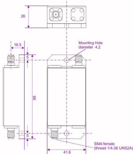
Fig. 10: Housing outline dimensions (millimeter)
