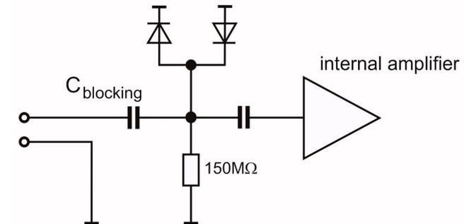
Fig. 6: Input protection scheme (each channel)
