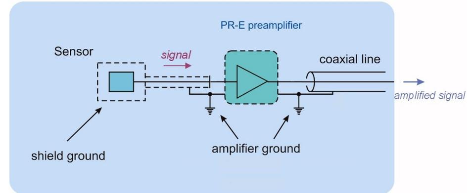
Fig. 5: Example of shielding and ground line
