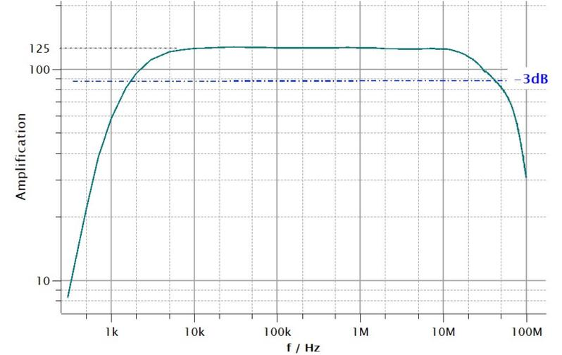
Fig. 8: Linear Voltage Amplification Factor vs. Frequency,  $T = 297$  K, with 50 Ohm load
