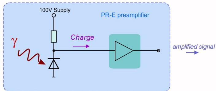
Fig. 1: Photon Counting Application with Avalanche Photo Detectors
