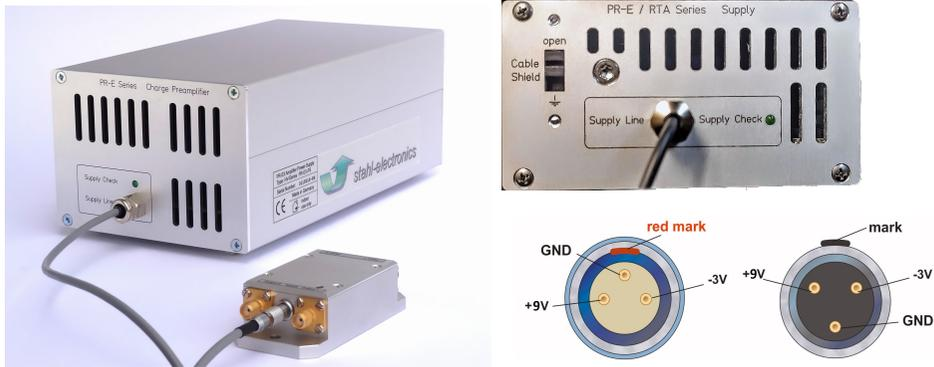
Fig. 4: Mains Supply, connection to amplifier module. Lower right picture: The Pin orientation as seen in the PR-E case outside, Lemo and XLR versions
