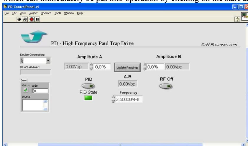
The device parameters may be entered in the corresponding numeric fields, after choosing the established COM-connection to the device and serial number (‘PD’ + last three digits).
