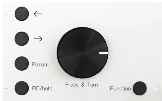
The device is manually operated by the control keys and the selection wheel. Pressing the button 'Param' selects the parameter to be changed. This button 'rotates' through the following parameters:
