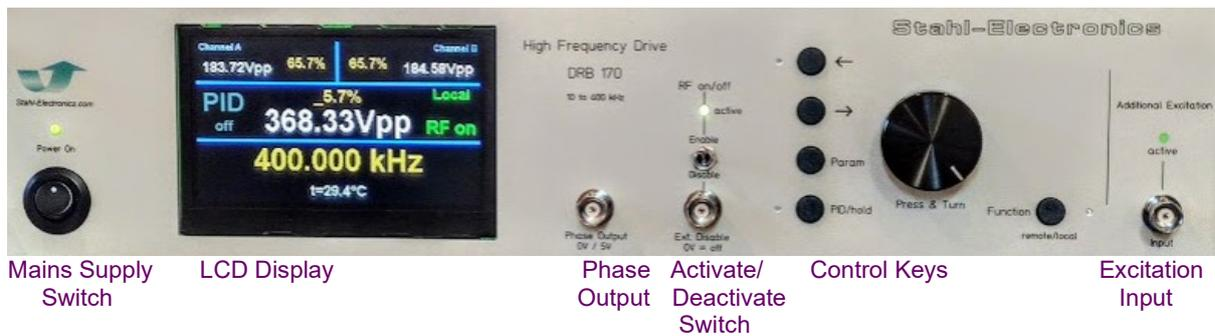
The front plate contains the main control elements of the device:
