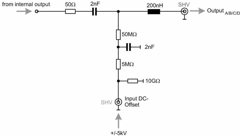
fig. A12: Circuit diagram of high voltage offset output stage. An externally supplied DC offset of up to  $\pm 5\text{kV}$  (max. value depends on rating) is filtered by a  $5\text{M}\Omega \times 2\text{nF}$  low pass and subsequently superposed to the AC signals from the internal phase shifter. Diagram shows one of four branches.
