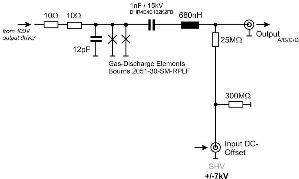
fig. A13: Circuit diagram of high voltage offset output stage  $\pm 7\text{kV}$  floating version. An external DC offset of up to  $\pm 7\text{kV}$  may be applied and is superposed to the AC signals from the internal phase shifter by means of a simple RC circuitry. Diagram shows one of four branches.
