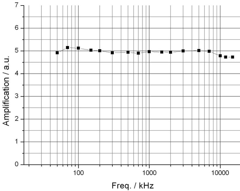
Fig. A8: Gain flatness vs. frequency
