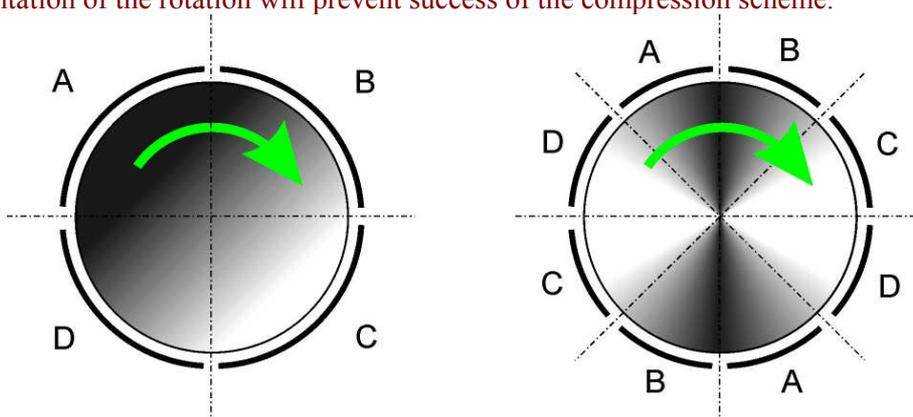
fig. 4.4 Graphical illustration of electric dipole/quadrupole creation. For a rotating electric dipole, connect the output lines (A,B,C,D) as shown in the left picture, for a quadrupole as shown in the right picture. Please observe the correct order while connecting the cables. The shading in the pictures above illustrates the momentary electric potential (dark: low; light: high).
