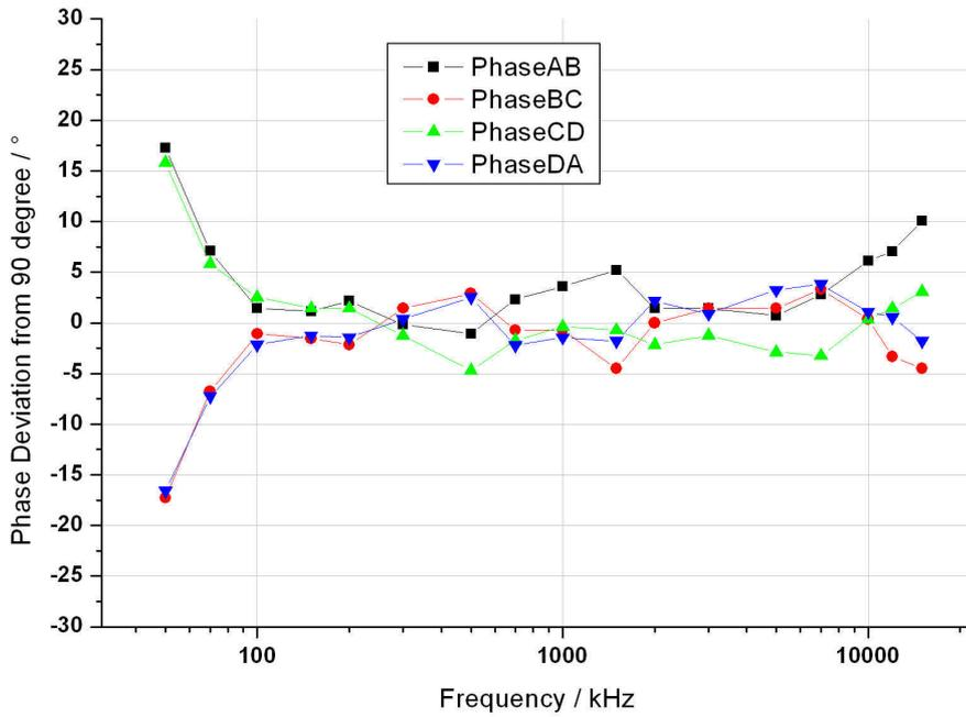
fig. A10: Phase error vs. frequency
