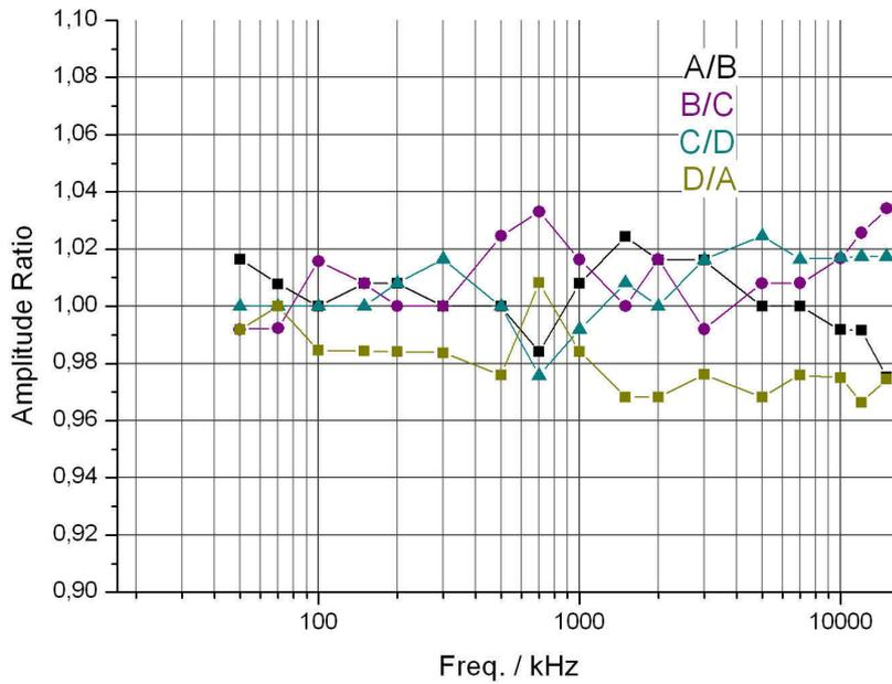
fig. A11: Typical amplitude mismatch vs. frequency
