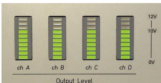
Note that the device must not be operated permanently at voltages exceeding the nominal value (10V<sub>pp</sub> or 100V<sub>pp</sub>).
